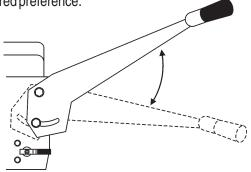
Figure 36. Handle Bar Height Adjustment
